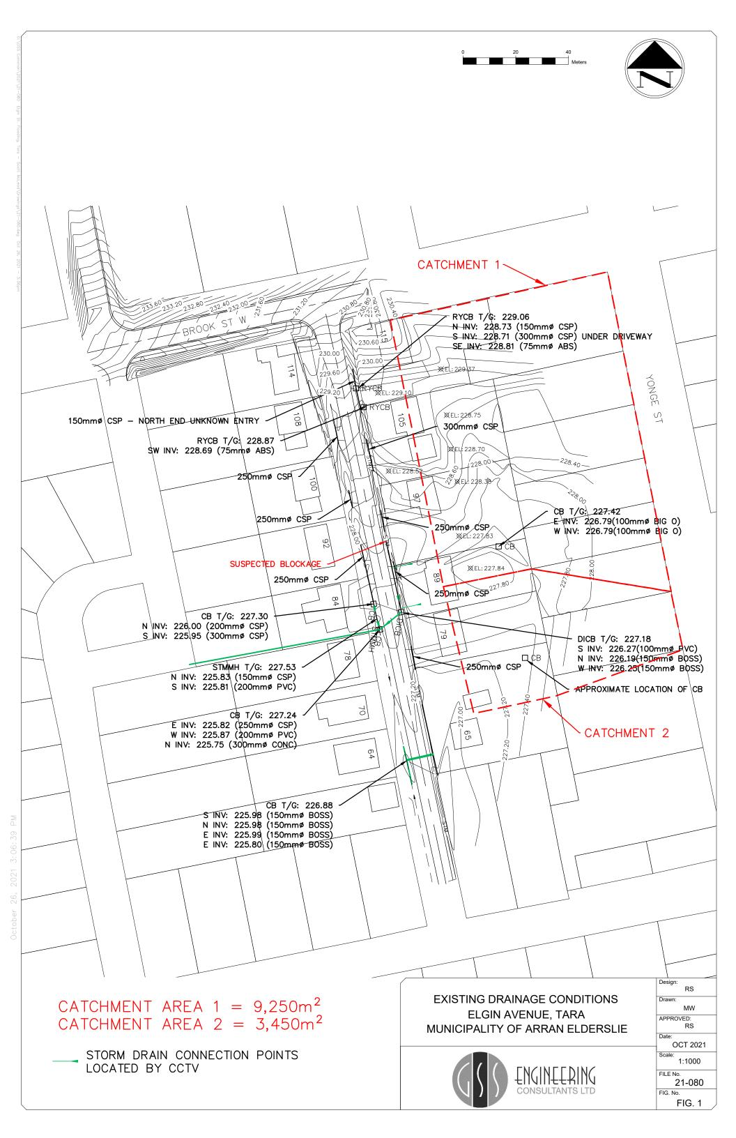
It was also noted that Elgin Street road profile creates a valley-like situation, where runoff collects at the lowest point near house #78 and #84 and drains towards the west by way of a 200 mm storm sewer. This storm sewer is deep but located potentially too close to house foundation.
