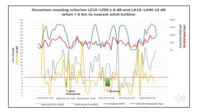
In contrast, this chart shows the conditions for the hypothesis test at the site > 6 km to the nearest wind turbines for the same week.. The blue turbine output and red wind speeds are identical to the last chart.
