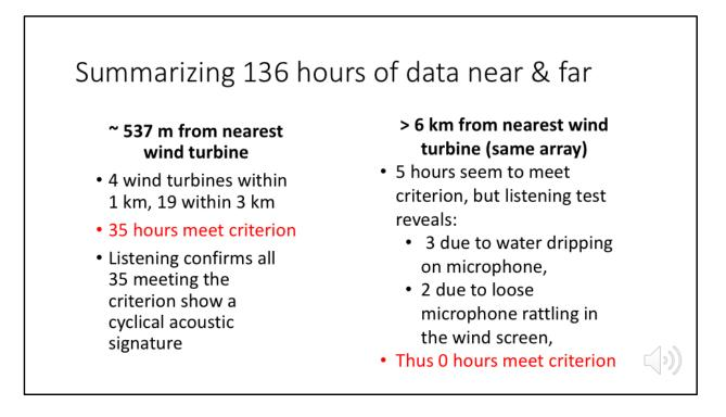
Summarizing, the 136 hours of simultaneous recordings near and far from the wind turbines, showed the following:
