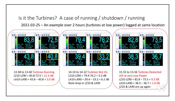
Here's an example of a shut down and restart at low power conditions. The left side shows the criterion test before the shutdown where (LZ10-LZ90=11.3 dB while LA10-LA90 = 3 dB). Just after the shut down, you can see the 7.6 dB drop in LA90 from turbines operating to shut down.
