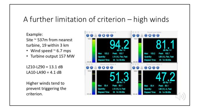
This slide shows a second condition that prevented the criterion from being met.
