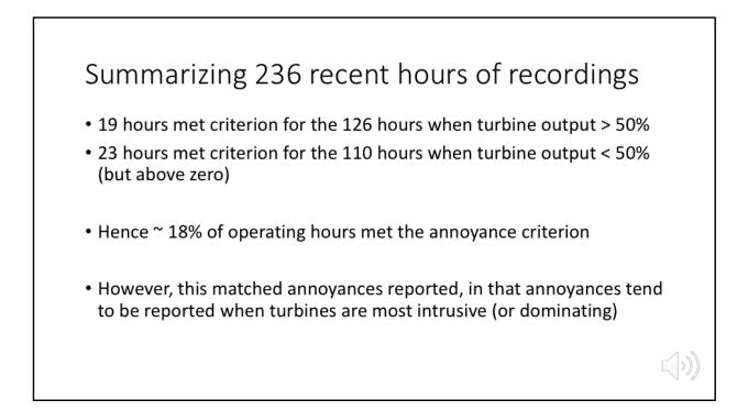
When we summarize the most recent 236 hours of recordings made at the home ~ 500 metres from the nearest wind turbine, we find that 19 hours met the criterion during the 126 hours when the turbine output was > 50%. During the 110 hours when the turbine output was < 50%, 23 of the hours met the criterion.
