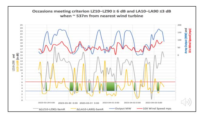
This chart shows the test to see if the proposed hypothesis was met during a week from measurements taken at the site  $\sim$  537m from the nearest wind turbine.
